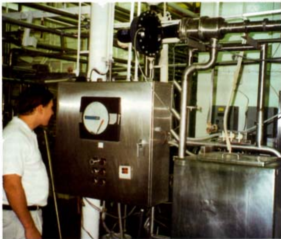
Direct contact steam injection allows companies to complete entire CIP cycles within considerably tighter time tolerances.
